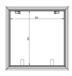
Dimensions passage = A3 – 32 mm x B3 Dimension vide de passage = dimension de montage A1 + 5-10mm x B1 + 5-10mm
