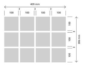
All dimensions in mm, (V) = locking side Order details: For dimensionally accurate customised production, please state the exact tile and joint dimensions when placing your order.
