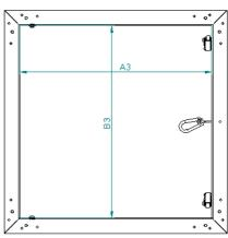
Clear opening dimensions = (A3 -14mm) x B3 Structure opening dimensions = installation dimensions (A1, A2) + (5 to 10mm)
